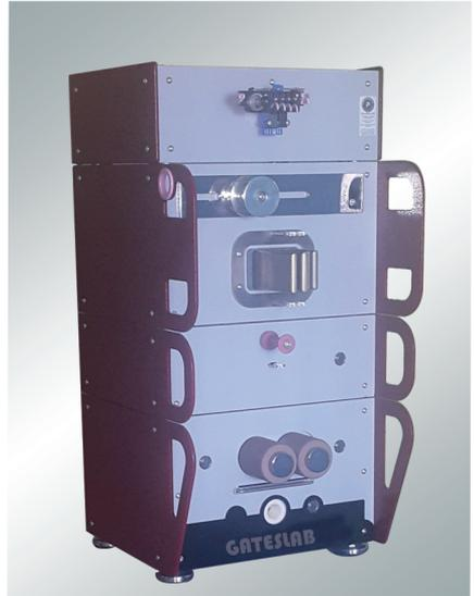
Device was designed to measure the variations of yarns, slivers, and rovings.
